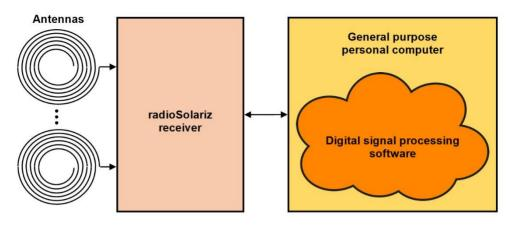
Fig. 1. RadioSolariz station general block diagram
