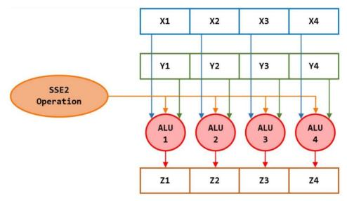
Fig. 2. Structure of streaming single instruction — multiple data extensions 2 operations on floating point 32-bit data
